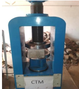
Fig 8 compression test for Brick
